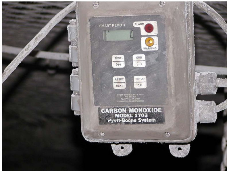
Photo 2. An example of the CO (carbon monoxide) monitors used to monitor the conveyor belt for mine gases underground at the Sago mine.
